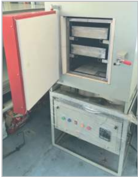
→ ELECTRICAL DUST BURNOUT FURNACE
