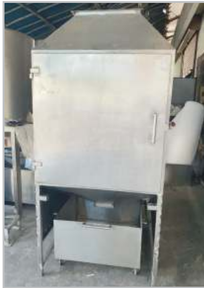
→ GAS DUST BURNOUT FURNACE
